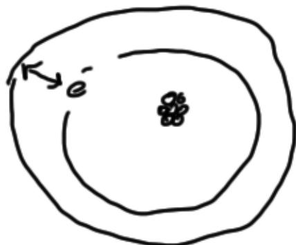
When the electron moves between energy levels it either emits or absorbs light
